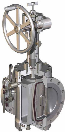
↑ GENERAL VALVE TwinSeal/TruSeal Double Block-and-Bleed Plug Valve Applications: Tank Farms, Meter Stations, Loading/Unloading, Multi-Product Manifolds, Hydrant systems and Fuel loading
